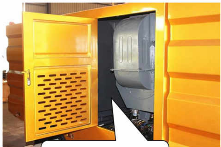
Open the side door to refueling the truck
